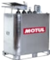
USED OIL CONTAINER FULLY EQUIPPED Complete used oil container with 995 l capacity for used oil AIII, double wall. Oil level display with full indicator and leak indicator, completely pre-mounted. Overflow safeguard, leak warning device, filling funnel, suction neck, vent neck and level display. w x d x h: 114 x 72 x 170 cm Comply with the specifications in the type approval and the VAWS (German Regulations on Facilities Handling Substances Dangerous to Water)/respective state regulations.
